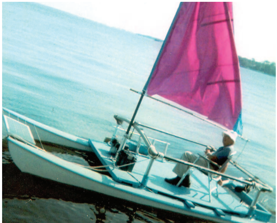
'47: John Corse at the helm of his converted Hobie Cat, showing a good view (in spite of the tilted camera angle!) of the solar panel between the bows, the new “old folks” deck and rail, the jury rig standby sail, the battery pack at its base, and the little outboard trolling motor
